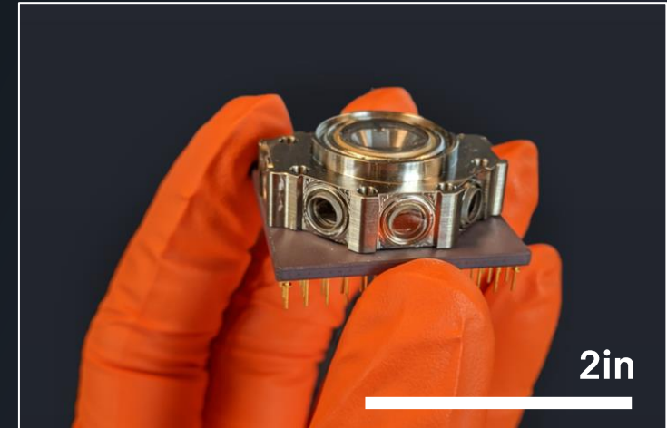
IonQ ion trap and vacuum chamber in a single, minuscule package 1
