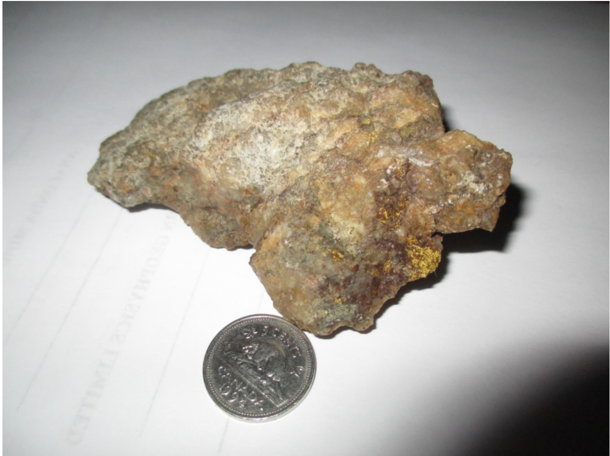
Plate 8: Coarse Gold Marginal to Quartz Veining, Deer Cove
