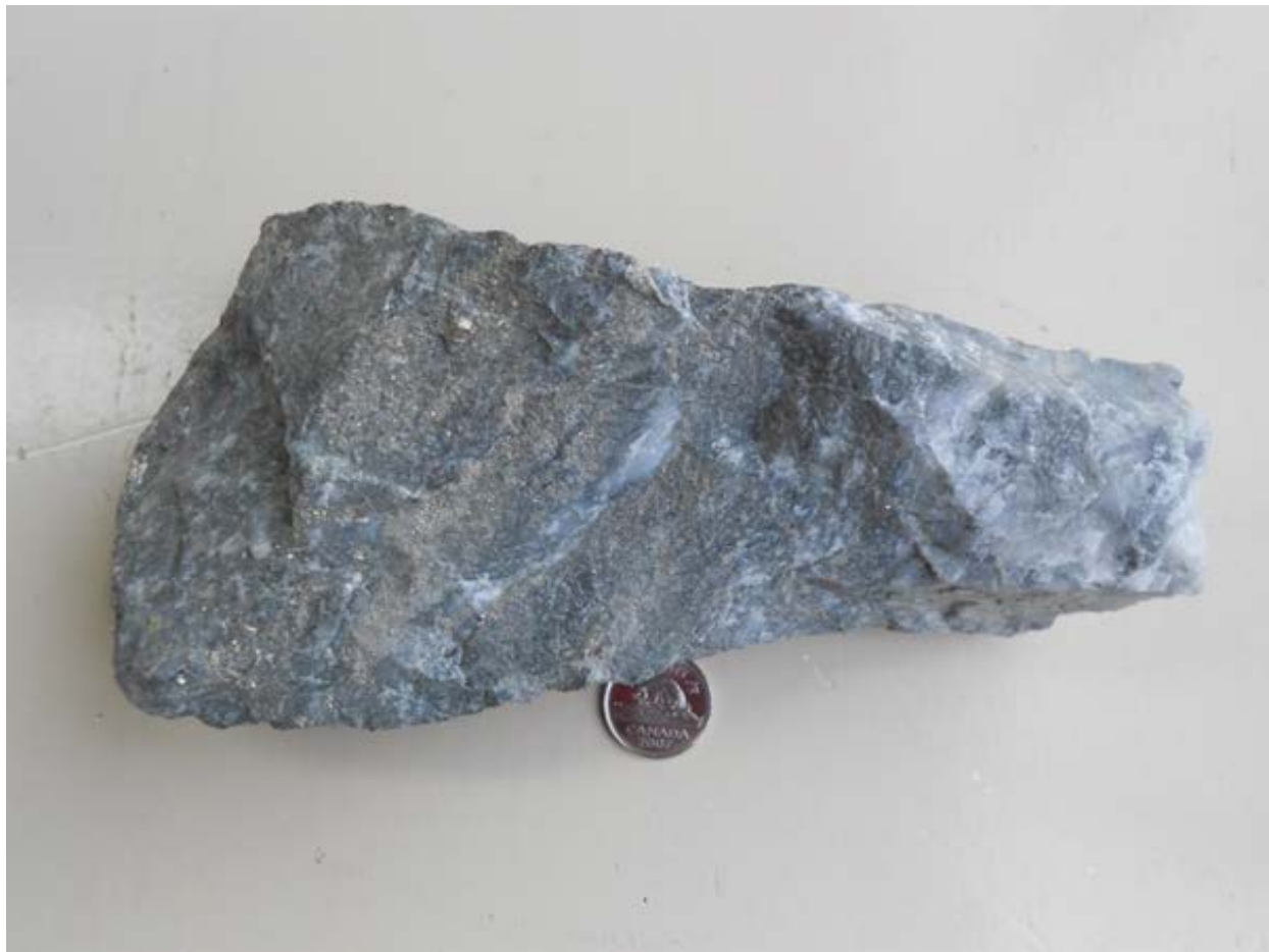
Plate 3: Typical High-Grade Ore (+2 g/t gold), Pine Cove Mine
