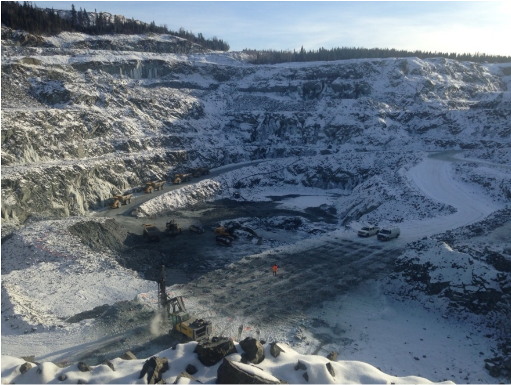
Plate 13: Pre-Blast Drill Pattern, Pine Cove Mine (2014)
