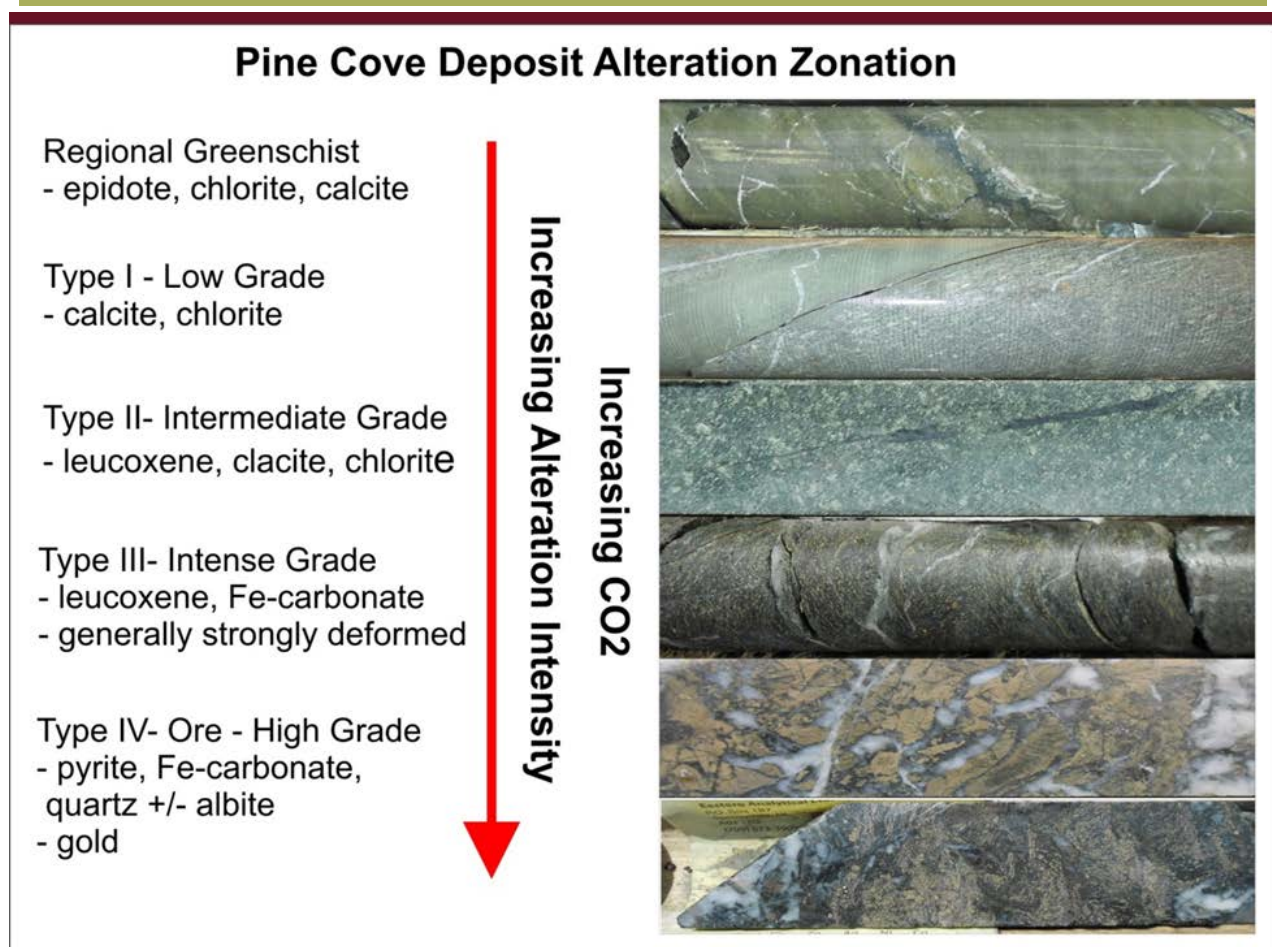
Figure 10: Alteration Zonation Associated with Gold Mineralization, Pine Cove Mine.
