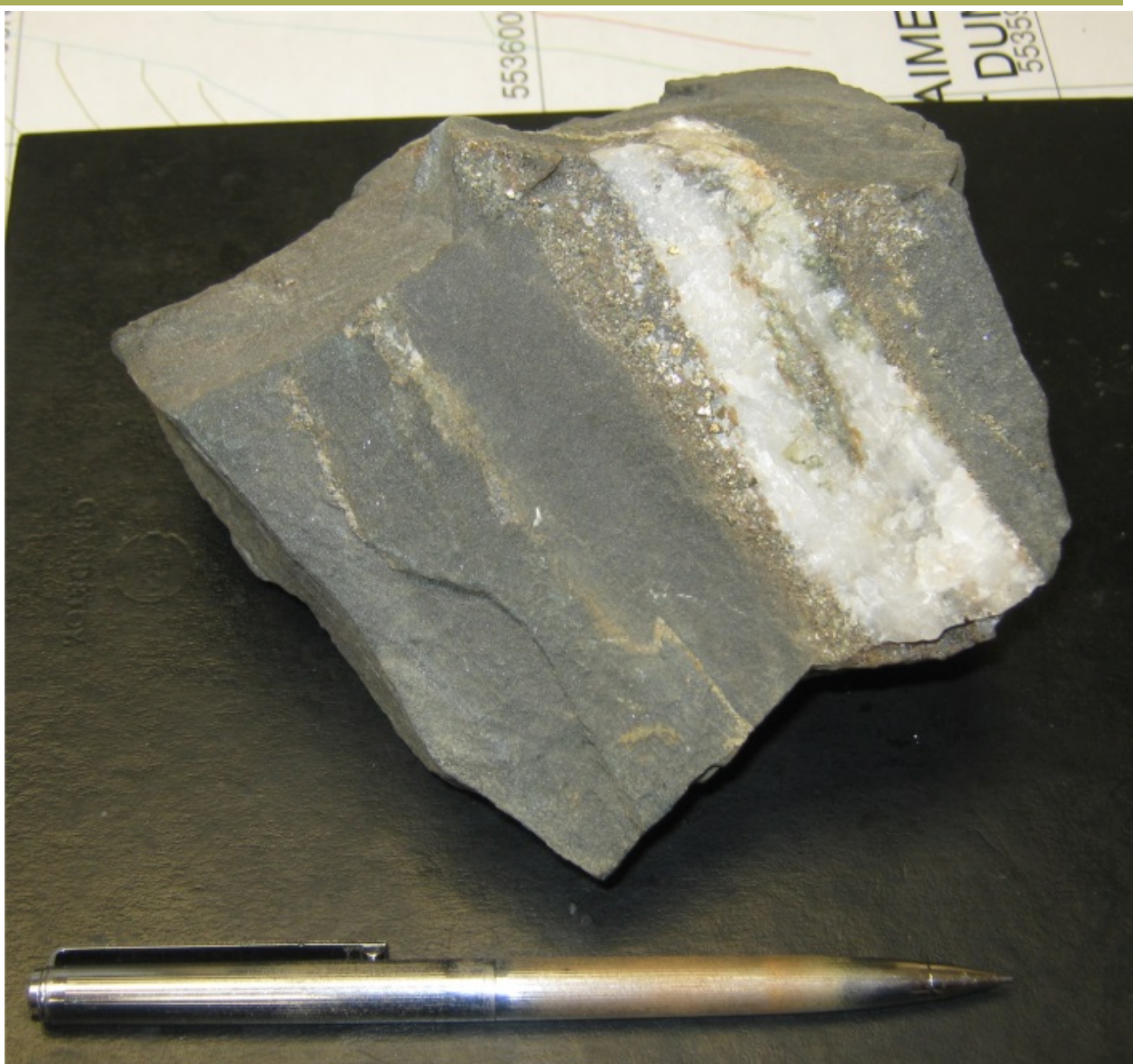
Plate 7: Grab Sample from Goldenville Mine Dump Showing Coarse Pyrite Mantling Quartz Veining Developed within Magnetite-Rich Iron Formation.
