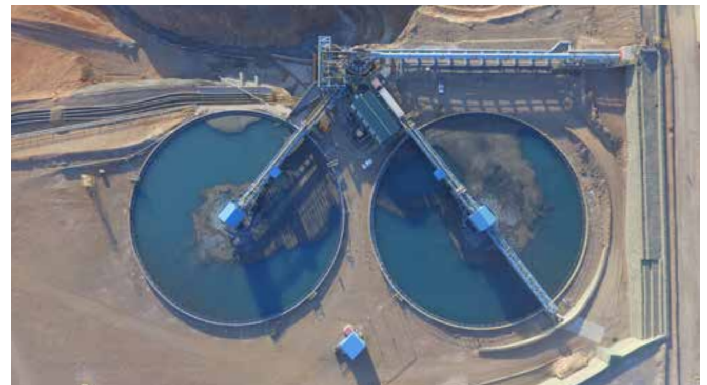
Aerial view of the water efficient tailings thickeners at Oyu Tolgoi
