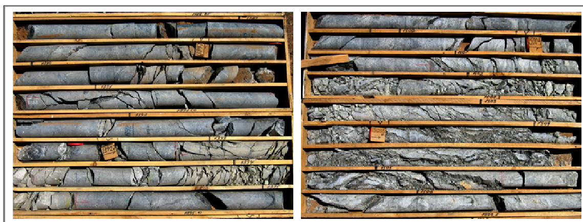
Figure 16.15 Localized Fractured Zone (left) and Large-Scale Fault Zone (right) from Drillhole EGD 104A (depth 1,330 m and 1,503 m)
