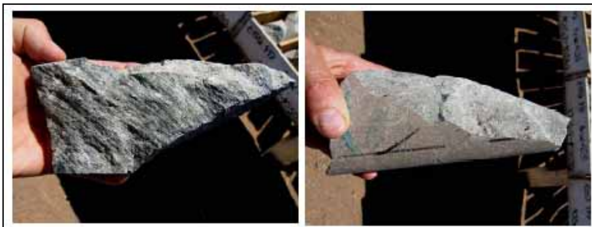
Figure 16.16 Slickensided but Undulating Joint and Rough Stepped Joint Surface Drillhole EGD 119, Approximately 1,030 mRL
