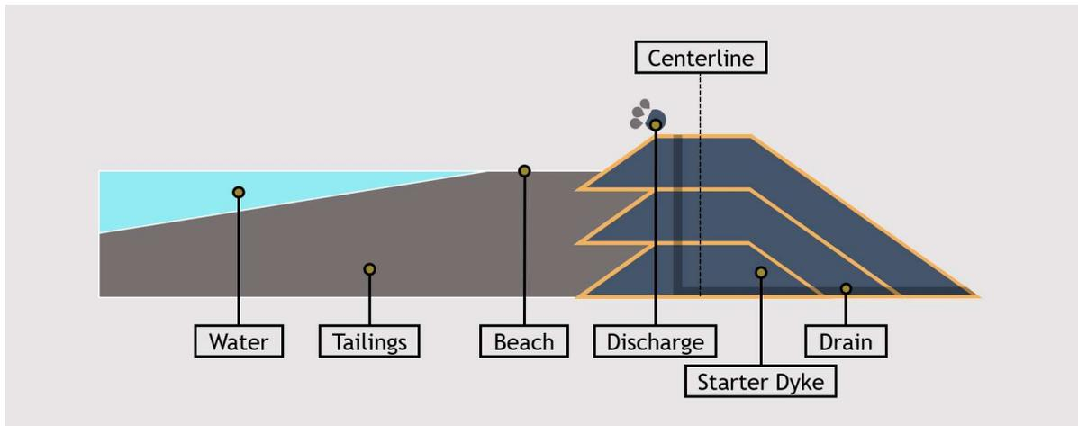
A centerline tailings dam is raised vertically and its construction combines the principles of both downstream and upstream design concepts. Similar to the upstream construction method, tailings are discharged behind each dam section and allowed to dry to form a beach. This tailings beach later supports the upstream slope of the successive embankment raise. Dewatering technologies such as thickening are commonly used to improve the construction of these structures.
