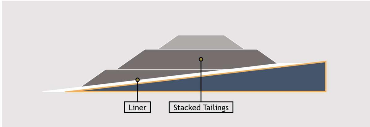
Following crushing, grinding and chemical leaching to separate the target mineral from the ore, tailings are dewatered in a plant, using a thickening tank followed by filters. Most of the process water in the tailings is recovered and returned to the plant for reuse in the processing of new ore material. The unsaturated filtered tailings, also known as filter cake, are deposited and compacted to form a stable dry stack.
