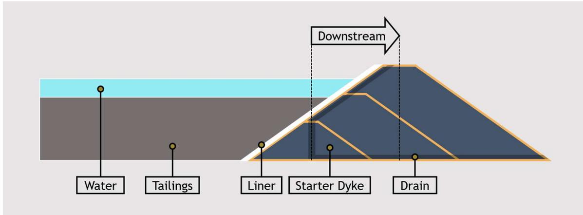
Downstream tailings dams resemble typical water retaining structures but are raised in stages during operations. Downstream tailings dams are raised following a downstream direction, starting at the starter dyke, and growing away from the initial impoundment area. Tailings slurry discharged behind each new section of the dam is not used to support successive raises of the dam.
