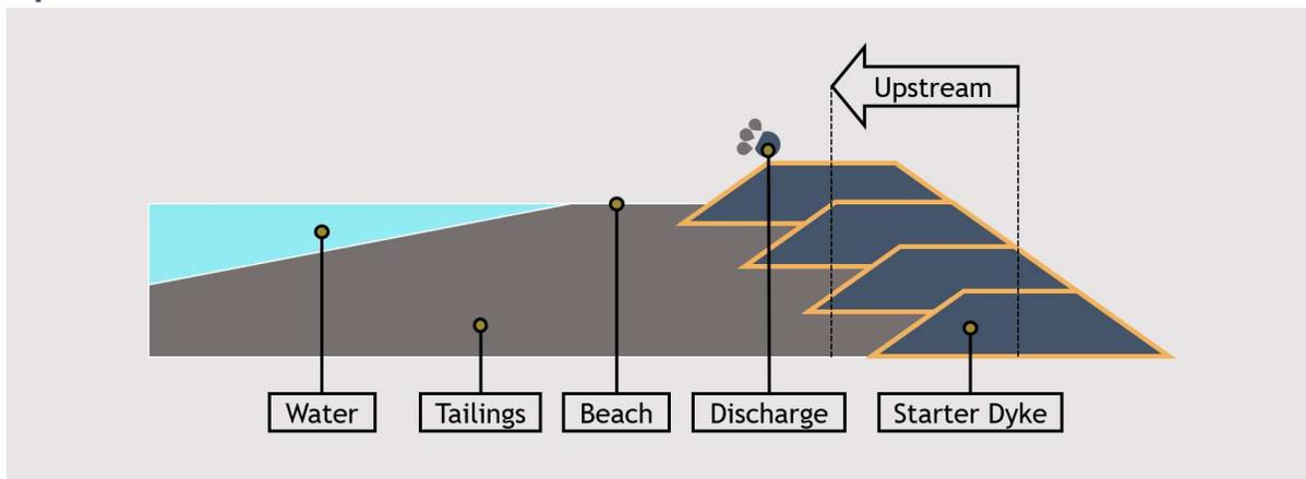
An upstream tailings dam is raised in the upstream direction of the starter dyke. Tailings discharged from the starter dike are deposited at an angle away from the dam crest and
