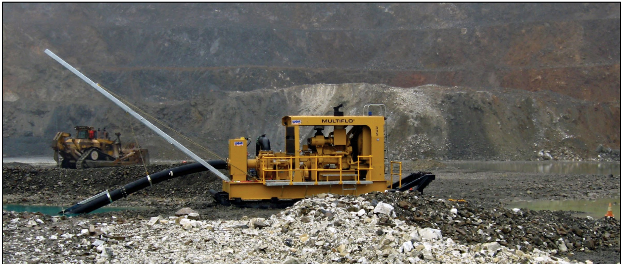
Figure 16-22: Typical Self-Prime Diesel Pump for Pit Sump
