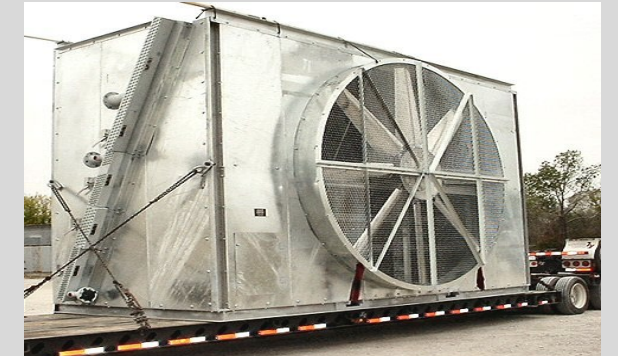
Air cooled heat exchangers (ACHX) for a data center
