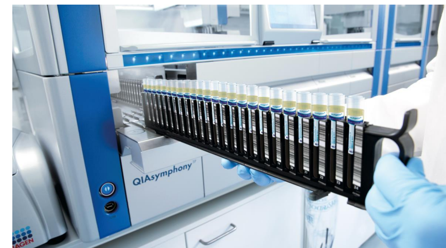
Liquid biopsy samples being loaded onto QIAsymphony
